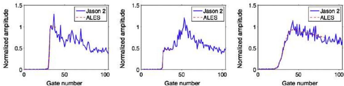
**Figure 3:** Example waveforms and their fits using the ALES retracker, from Passaro et al. (2014)
